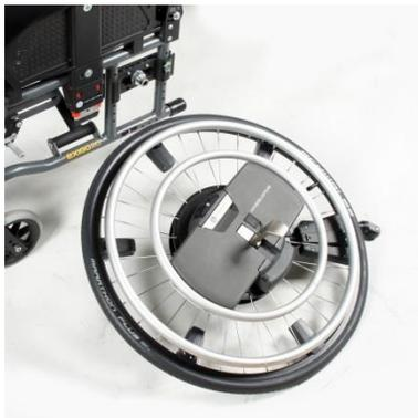
If you push the small drive rim slightly forward (or backwards), you move with continuous drive – no self-propelling required. Switch between both rims as needed. The WheelDrive wheels can be quickly removed from your wheelchair for easy transport. The integrated batteries can be charged on-wheel or disconnected and charged separately.
