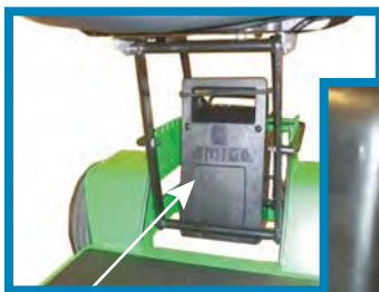
Spare battery under seat
