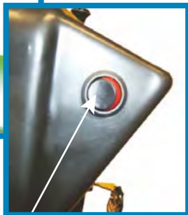
Speed range switch: High speed range 0-4 mph (0-6.4 kph) Low speed range 0-3 mph (0-4.8 kph)
