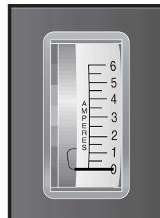
Figure 9. Ammeter Indicates Batteries Are Fully Charged
