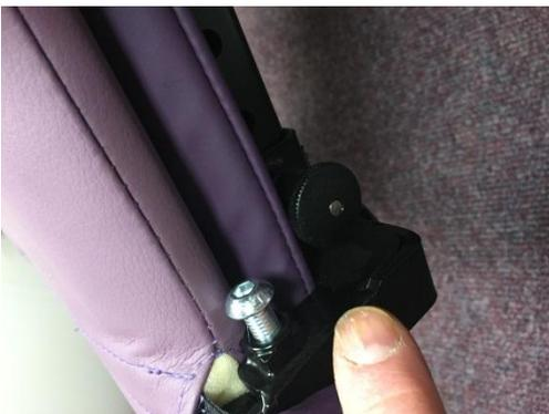
To adjust the height of the footplate the index plunger pins on both sides need to be pulled out and the footplate can be positioned higher or lower in line with the next set of holes.
