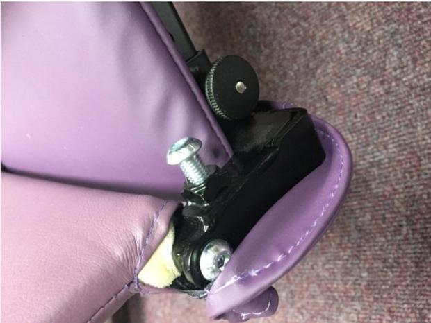
The angle of the footplate can be adjusted using the chromed dome bolts highlighted. It is possible to adjust the angle from -10 degrees to + 20 degrees
