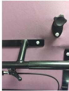
There are two knobs on the back of the chair which allow the carer to change the angle of the upper part of the backrest to give more head support or allow for a kyphotic curvature of the spine.
