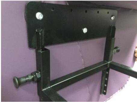
To adjust the height of the arms release both plunger pins simultaneously and move the arm to the desired height.
