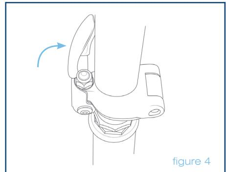
6. Insert seat post into seat receptacle on frame. Set to desired height and secure in place by inserting thumb screw and turning clockwise until tight.
