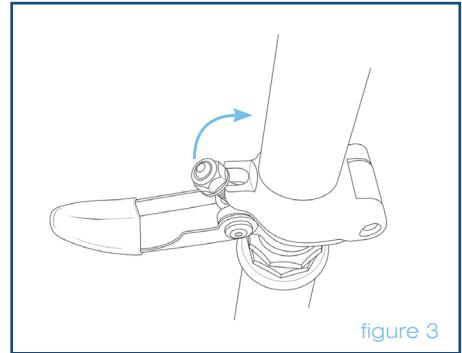
5. Secure screw and tiller in place by pushing locking handle against the side of the tiller (figure 4).
